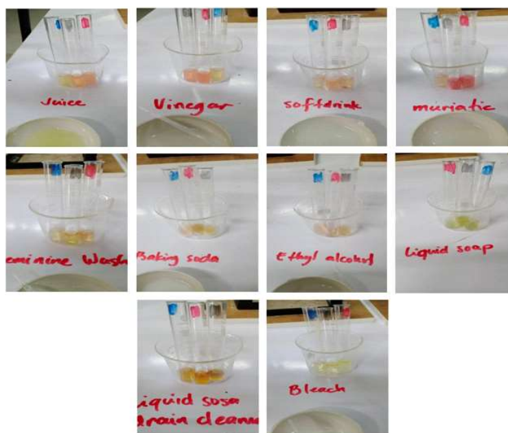
Figure 2. Household chemicals with natural acid-base indicators. Label: blue= C. blumei , gray= C. ternatea , pink= A. catechu
