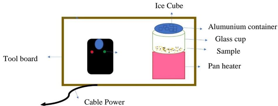
**Figure 1.** The design of the sublimation tool
