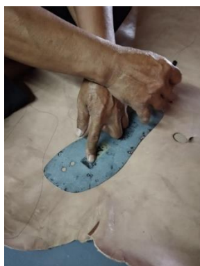
Gambar 1 Proses Memola Diatas Kulit (Sumber: Nawawi, 2023)
