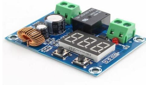
Gambar 3. Modul low voltage disconnect
