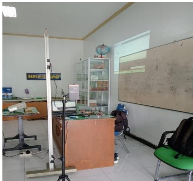
Figure 3. Free fall motion kit adruino and phyphox application
