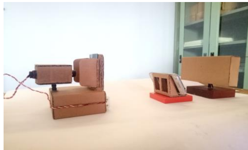
Figure 2. The simple light diffraction teaching aid
